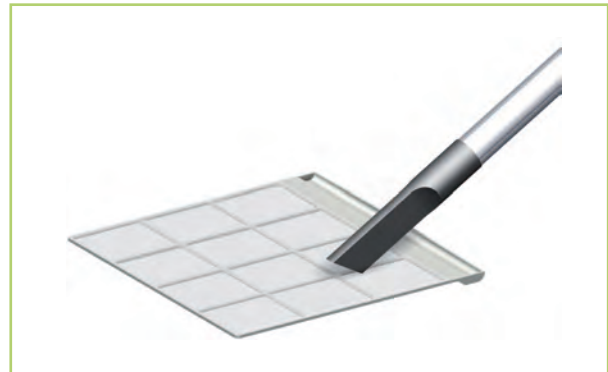
Fig. 16: Cleaning with a vacuum cleaner
